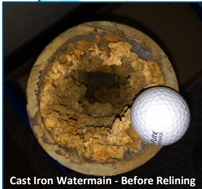
Cast Iron Watermain - Before Relining
