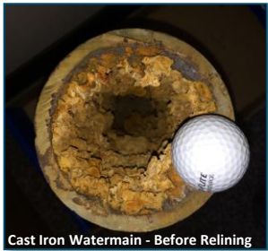
Cast Iron Watermain - Before Relining
