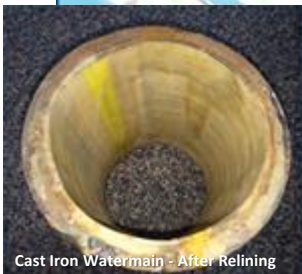
Cast Iron Watermain - After Relining
