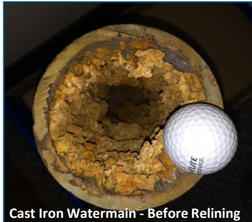
Cast Iron Watermain - Before Relining
