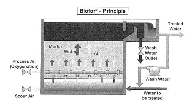
Aerated biological filtration combines in a single step both biological degradation of biodegradable soluble matter and solids retention by mechanical filtration of suspended solids. Clarifier downstream is not needed.
