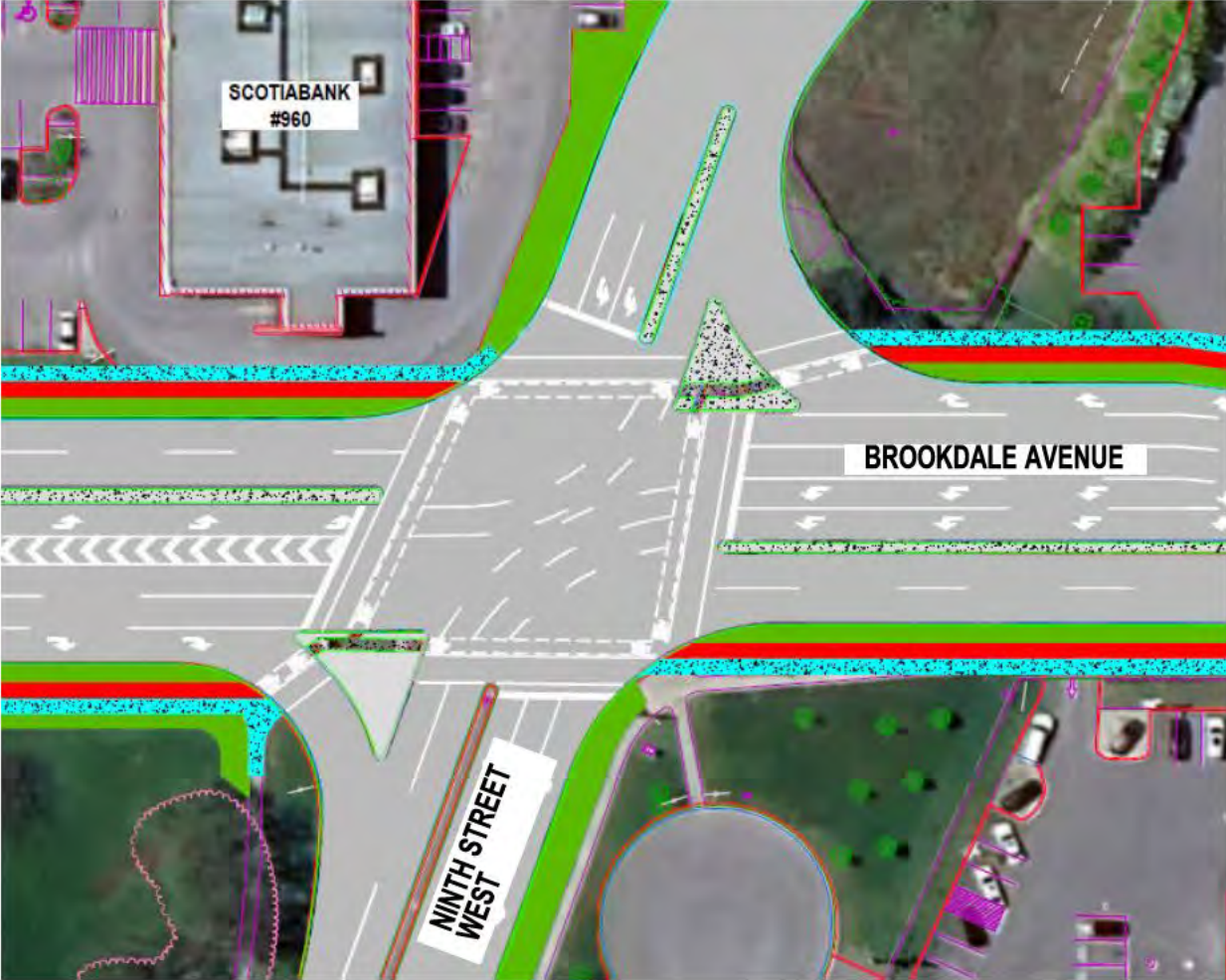
Right-turn Channels Maintained
