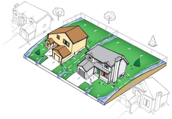
Proper lot grading and drainage is important to ensure surface water flows away from a building's foundation to a suitable outlet. Improper lot grading can result in ponding, settlements, basement dampness, insurance claims and conflicts between owners of neighbouring properties.
